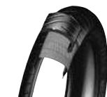
BELTED TYRE WITH RADIAL CARCASS (90 DEGREES)
