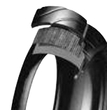
0° - STEEL BELTED TYRE WITH RADIAL CARCASS (90 DEGREES)
