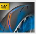
What is it? Optimised front tyre heat control achieved through intricately calculated tread groove pattern and footprint
