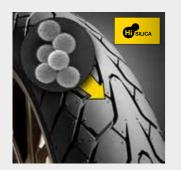
What is it? Compound blend combining wet grip resin in the shoulder compound with a very high silica ratio
