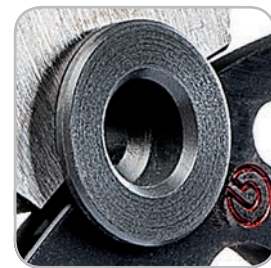
Trascinamento a bussola tonda. Round bushing drive system.
