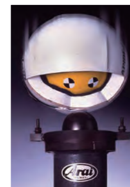
All helmets protect the rider's head through both glancing off and energy absorption.
